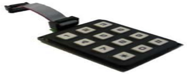
Fig.5: Keypad interfaced with microcontroller
